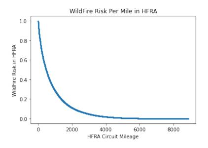
The horizontal axis in the figure represents the cumulative circuit mileage in the HFRA, and the vertical axis represents the sum of all the wildfire risk in terms of both probability of ignition and consequences for circuit segments in HFRA.
