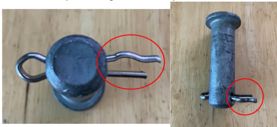
Figure 1: Properly installed clevis pin and cotter key (SAP 10068322)
