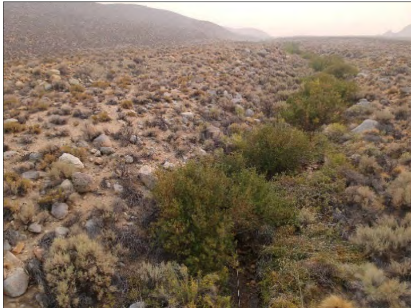
Photo 4.2-1 Transect Tape in Centerline of Stream Channel to Guide Placement of Transect Locations
