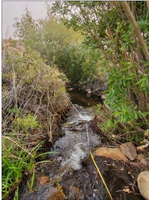
Photo 4.2-1 Transect Tape in Centerline of Stream Channel to Guide Placement of Transect Locations
