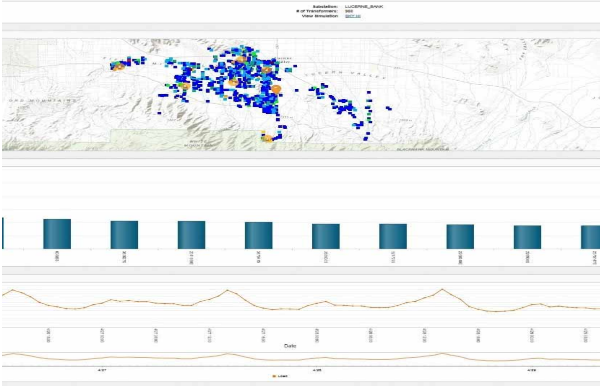
Figure 7, Transformer Dashboard Map overlaid on electrical distribution network GIS to visually identify all transformers
