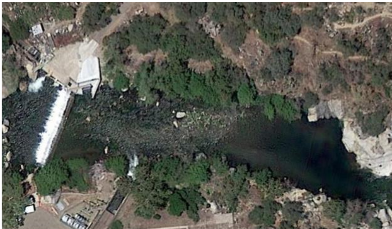
Figure AQ 5-2b. An image of the Kaweah No. 2 Diversion pool sediment deposit (Google Earth image).
