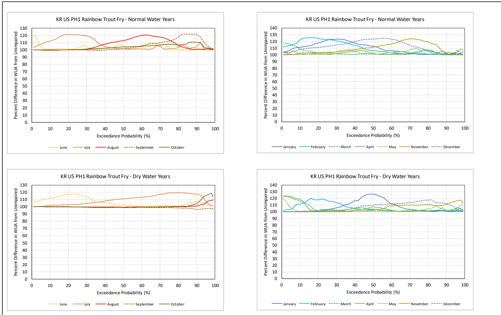
Figure B8.4-13. Kaweah River Downstream of East Fork Kaweah Confluence and Upstream of Kaweah No. 1 Powerhouse Rainbow Adult Fry Percent of Unimpaired Habitat Exceedance Plots (1994-2018) for Normal (top) and Dry Water Year Types (bottom) (warm water temperature months, left, cool water temperature months, right) using Proposed Action Minimum Instream Flows
