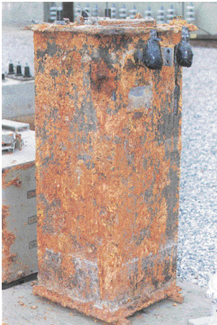
Figure 5–4: Heavy Corrosion — Example 1 of 3
