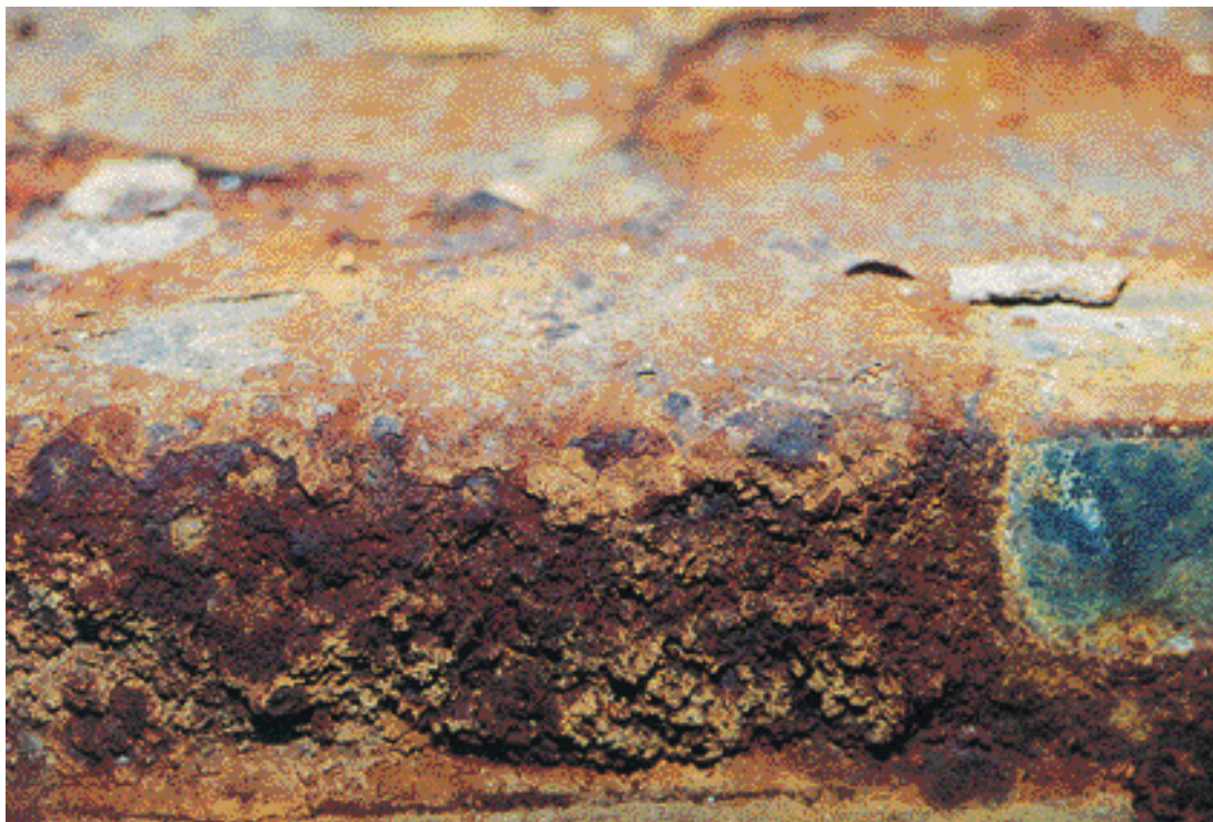
Figure 5–8: Moderate Corrosion — Example 2 of 3
