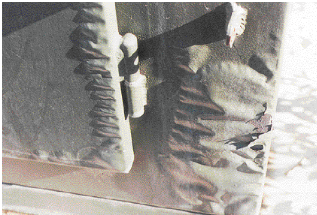
Figure 6–13: Significant Blistering of Paint
