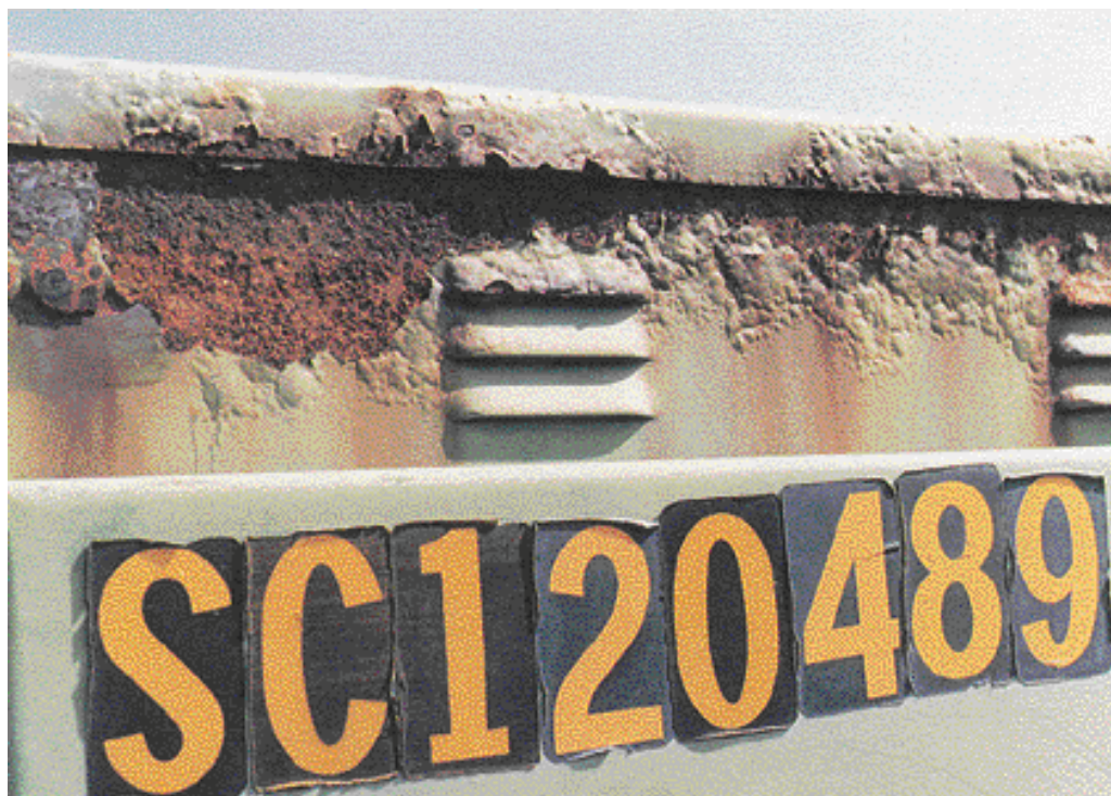
Figure 6–6: Pitting Exceeding One-Quarter Depth of Wall Thickness
