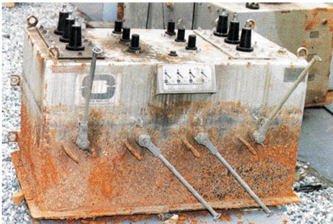
Figure 5–10: Light Corrosion — Example 1 of 3
