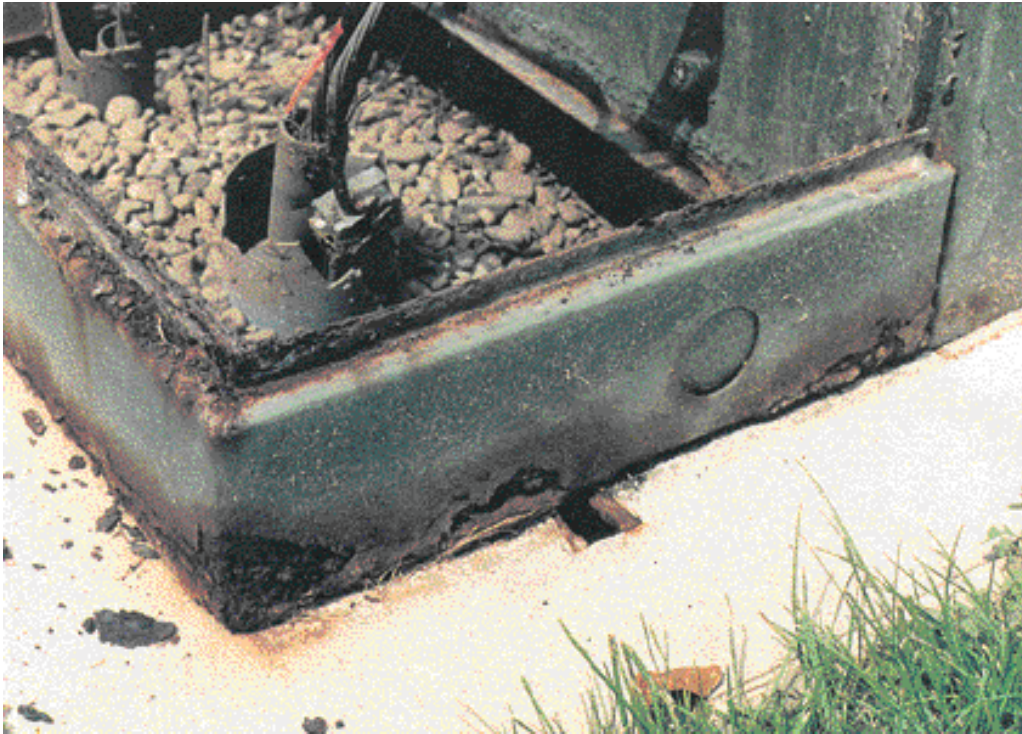
Figure 6–11: Another Example of Heavy Corrosion with Deep Pitting, Exceeding One-Quarter of Original Wall Thickness
