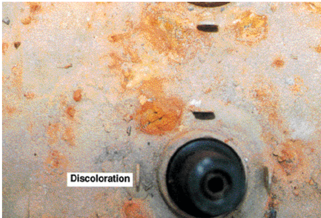
Figure 5–12: Light Corrosion — Example 3 of 3
