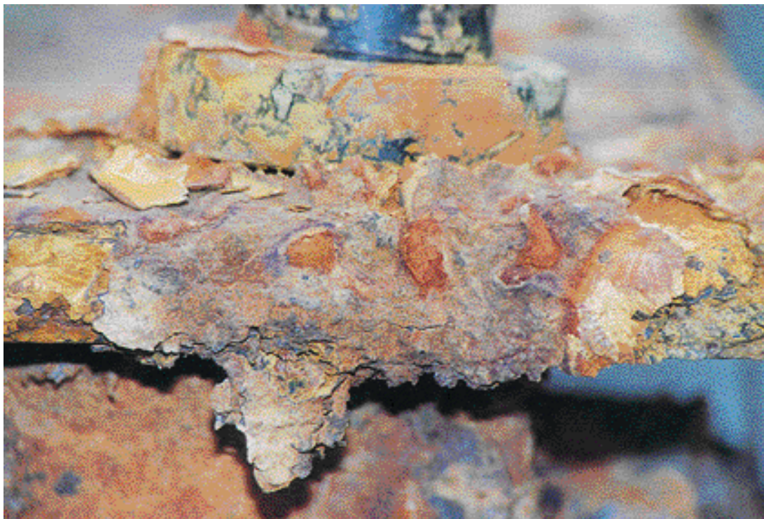
Figure 5-5: Heavy Corrosion — Example 2 of 3
