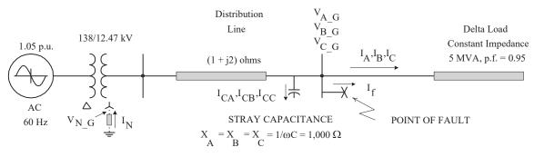
Figure 11—A typical distribution system with a radial feeder
