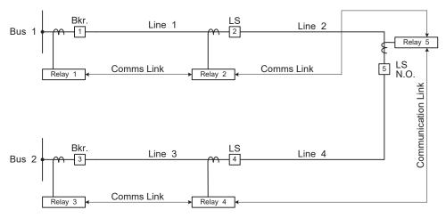
Figure 53—Communications-enhanced trip and restore scheme on a looped-radial distribution system
