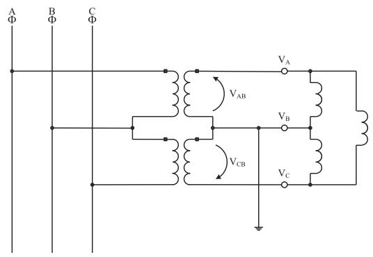
4 Figure 38—Three-phase, three-wire (open delta) connected VTs
