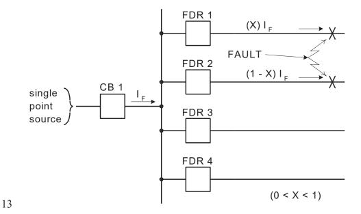
Figure 48—Faults involving two circuits
