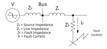
Figure 1—Fault on radial system
