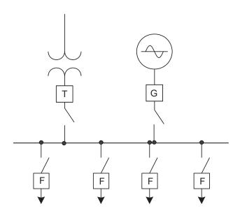
Figure 18—Generator connected to distribution substation bus
