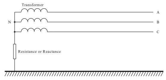
Figure 10—Resistively or reactively grounded system
