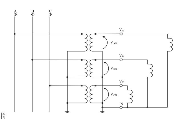
Figure 37—Three-phase, four-wire connected VTs
