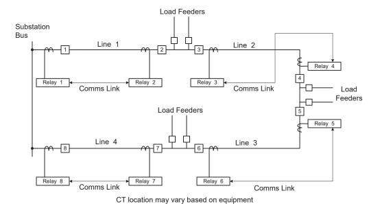
Figure 54—Example of a Communications-aided trip scheme on a closed loop distribution system
