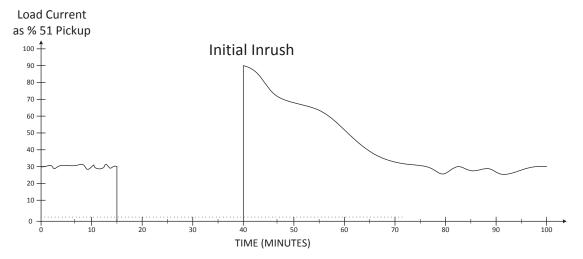
Figure 47—Cold load pickup
