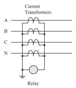
Figure 20—Ground relay and residually connected CTs
