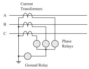
Figure 19—Typical phase and ground relay connections
