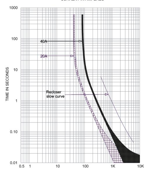
Figure 36—Time-current curve showing fuse blowing scheme
