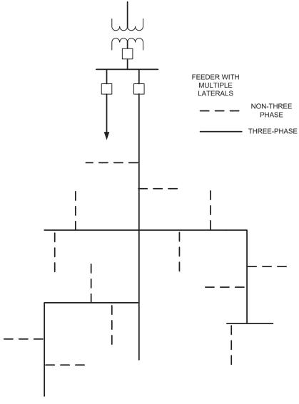
Figure 62: Example of a Distribution Feeder Structure
