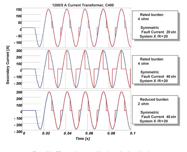
Figure 30—CT saturation at rated burden and reduced burden
