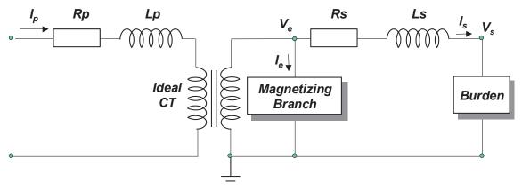
Figure 28—CT equivalent circuit
