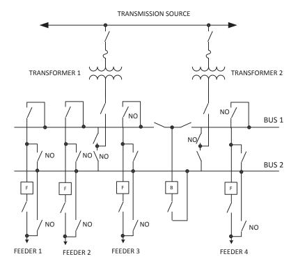
Figure 17—Dual-operation bus with two transformers
