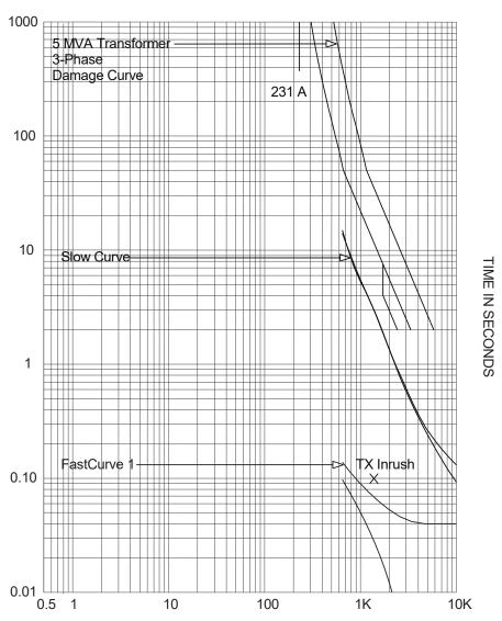
Figure 41—Coordination with large transformer with possible trip on inrush point at 1389 A
