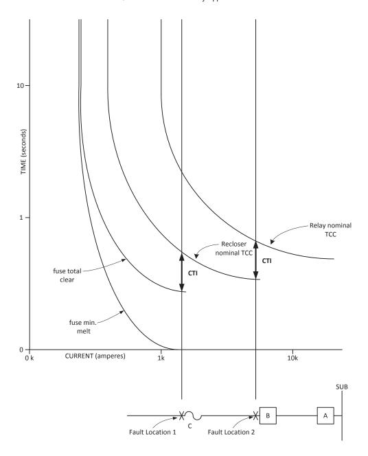
Figure 43—Coordination using a Coordination Time Interval (CTI)
