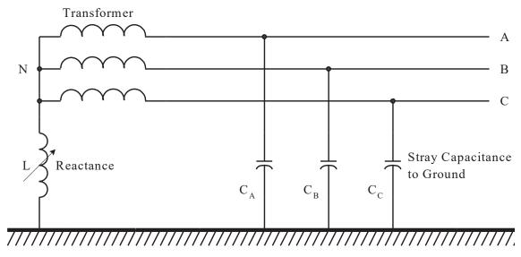
Figure 7—Resonant-grounded system
