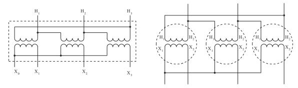
Figure 24—Three-phase and single-phase transformer connections
