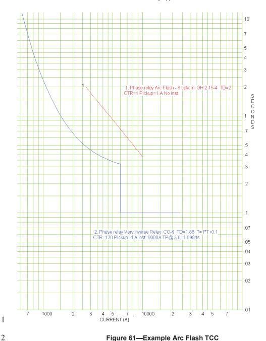
Figure 61—Example Arc Flash TCC
