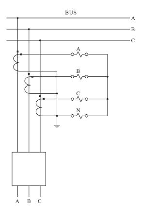
Figure 26—CT connection, 3-wire
