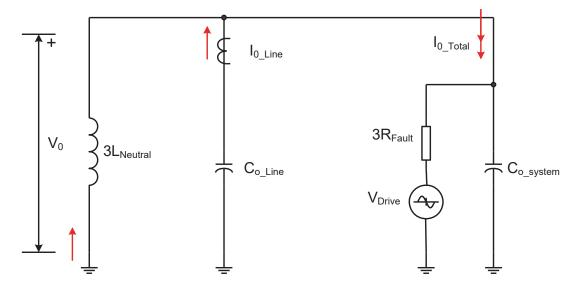
Figure 58—Zero-sequence network diagram for a reverse fault
