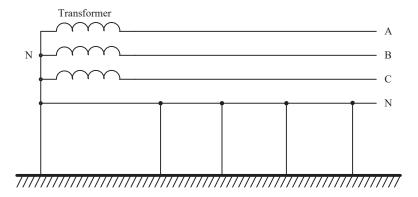
Figure 2 - Four Wire Multi-Grounded System
