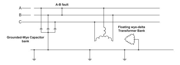
Figure 56—Ungrounded system where ferroresonance could occur
