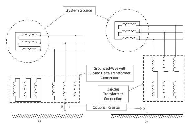
Figure 23—Grounding transformers
