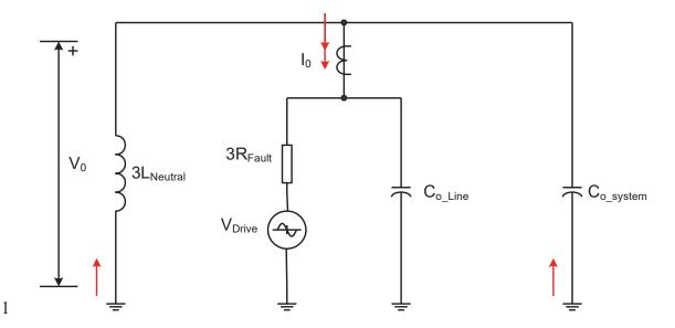
Figure 57—Zero-sequence network diagram for a forward fault
