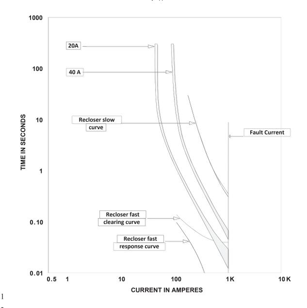
Figure 34—Time-current curve showing fuse saving scheme
