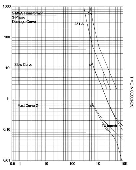
Figure 42—Coordination with large transformer with minimal possibility of trip on inrush point at 2315 A
