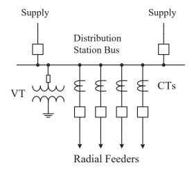
Figure 25—CT and VT location in a distribution station
